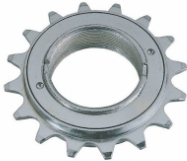
VI-211 FREEWHEEL 16T. SINGLE SPEED Available in 1/2" x 1/8", 24 TPI BSCY / 1mm pitch threads. (Available in Both Half & Full Balls)
