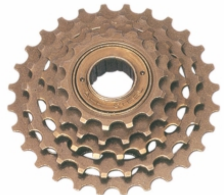
VI-216 5 MULTISPEED FREEWHEEL Teeth 14 to 22 or 14 to 28 Chain 1/2" x 3/32" Thread 34.80 x 24 TPI
