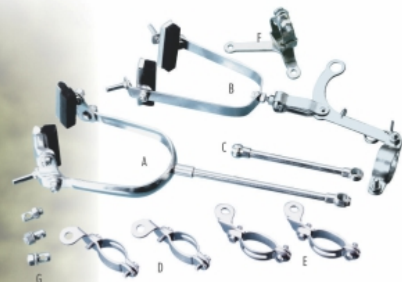
VI-395 BRAKE SET BALLOON TYPE (A) Front Stirrup with Tube & Brake Shoe. (B) Rear Stirrup with Adjustable Bolt & Bottom Leg Unit with Clip & Spring. (C) Rear Brake Tube with Screw. (D) Brake Clip Front with Screw & Nut (E) Brake Clip rear with screw Nut (F) Clip fastening "L" shape bag ball crank lever (G) Brake Button with Nut & Washer (H) Rear Brake Long Connecting Rod
