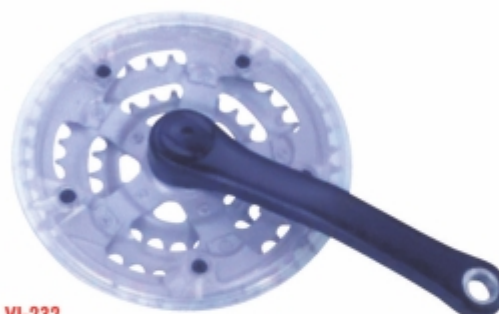
VI-232 TRIPLE CHAINWHEEL INDEX TYPE For 1/2" x 3/32" Chain. Available in 28/38/48T or 24/34/42T x 170mm Chainwheel Silver Grey With Plastified Crank Without Spider Crank Black or Grey With or Without Chain Guard, Transparent Guard.
