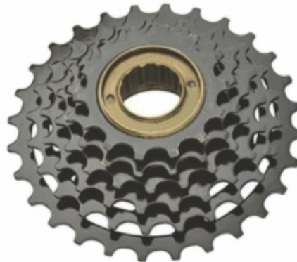
VI-215 6 MULTISPEED FREEWHEEL INDEX TYPE Teeth 14 to 24/26/32 Chain 1/2" x 3/32" Thread 34.80 x 24 TPI
