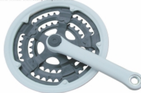
VI-234 TRIPLE CHAINWHEEL INDEX DARK GREY 24/28/34/38/42/48 Grey Plastified 170 MM Silver Grey with Plastified Crank with or without Chain Guard For 1/2" x 3/32" Chains.
