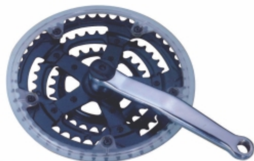
VI-233 TRIPLE CHAINWHEEL SSS INDEX For 1/2" x 3/32" Chain. 28/38/48 or 24/34/42T x 170mm Fish Type BCP Steel Crank or Powder Coated Black with Transparent Guard.
