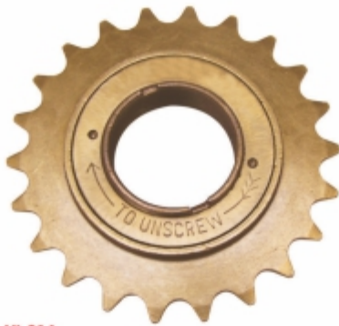
VI-214 FREEWHEEL 22T. SINGLE SPEED Single speed 18T, 16 T. Available in 1/2" x 1/8", 24 TPI BSCY / 1mm pitch Threads. (Available in Both Half & Full Balls)
